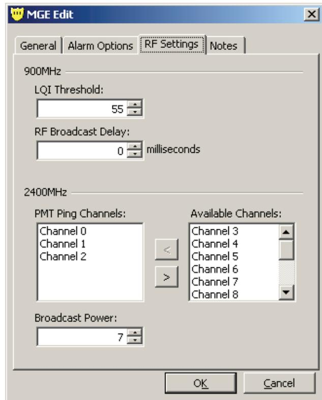
**LQI Threshold:** Link Quality Indicator. This value sets the minimum strength at which an MGE will continue to connect to a field device. The default value is 55; a range of values between 1 and 255 is possible. A value of 75 or higher is recommended.
