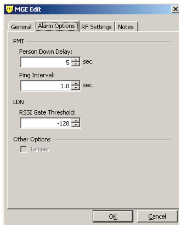
**Person Down Delay:** This sets the delay that the HDT will experience (with warning tones) once a man down condition is experienced. The default value is 5 seconds, available values are 1—255 seconds.
