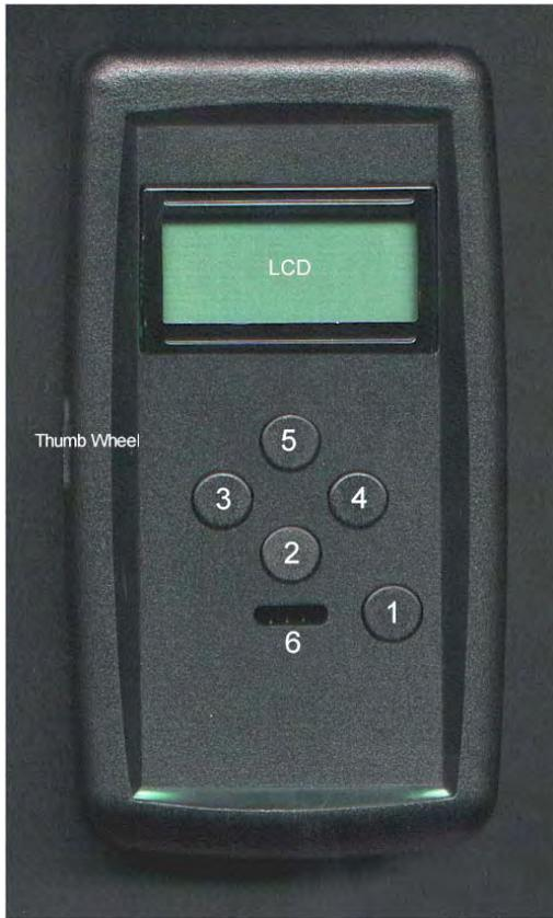
The 60703 is used to program IRTs with their ID value and to verify that programmed units are transmitting the correct value. Values are displayed on the LCD readout, and navigation is accomplished via the five buttons and thumb wheel. A 3-pin programming output is available for attaching the programming cable. The 60703 is powered by one 3V Lithium battery (CR123A)
