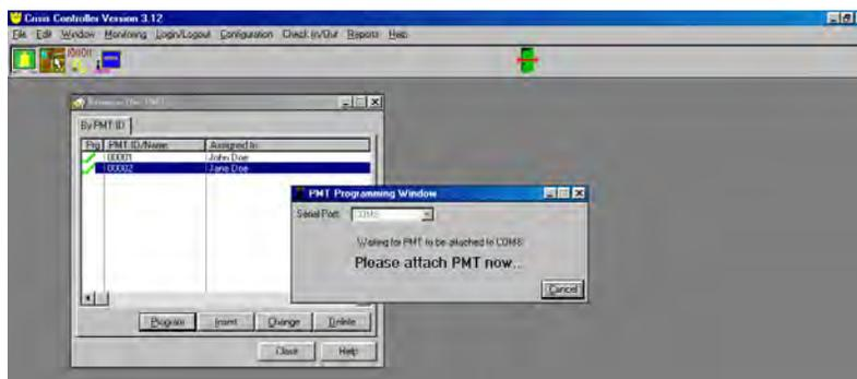
A message will appear stating **Please attach PMT now**. Connect the PMT to the programming cable stereo jack.
