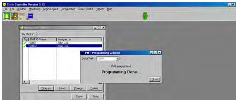
Once the PMT has been programmed correctly, a message will appear on your screen stating **Programming Done**. Disconnect the PMT from the programming cable.
