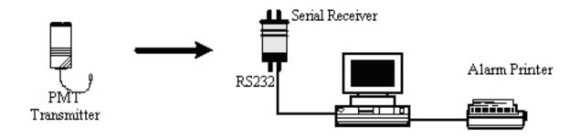
The Serial Receiver is connected to the Alert Monitoring Center via an RS232 interface. The Crisis Controller©™ software displays the alarm data (including location, user identification and alarm type) and shows the location on graphical maps tailored for your facility. Received alarms can be manually or automatically acknowledged and reset. The software also includes functions for device supervision and system configuration.
