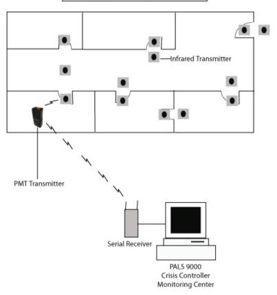
Although Infrared is a line of sight technology, the manner in which ASP utilizes this technology greatly mitigates the possibility that a Locator ID will not be read. Once the PMT sees an IRT Locator it stores the location code and does not require additional contact with the IR device. The stored location information is transmitted via RF to the Monitoring Station, ensuring accurate alarm receipt. This is fundamentally different that other IR systems that do require constant IRT contact.
